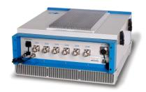
Upon activating Mobile Signal Jammer, all idle phones will indicate "NO SERVICE". Incoming calls are blocked as if the cellular phone is OFF. When Mobile Signal Jammer is turned off, all cellular phones will automatically re-establish communications and provide full service.
